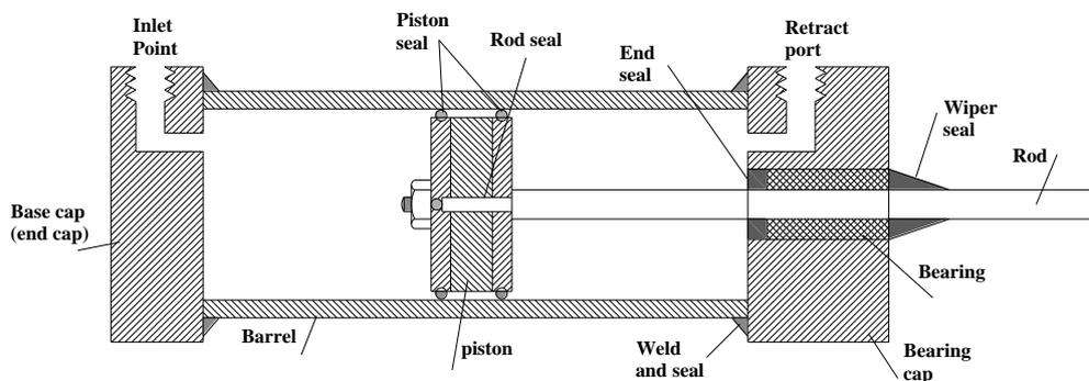
Figure 1.7 Construction features of double acting cylinder
