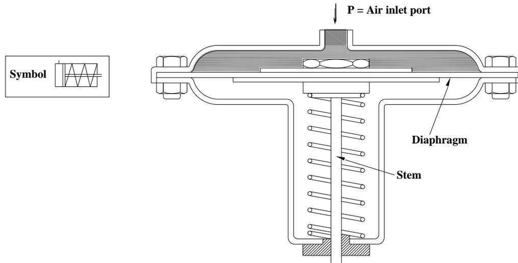
**Figure 1.2** Construction features of diaphragm cylinder
