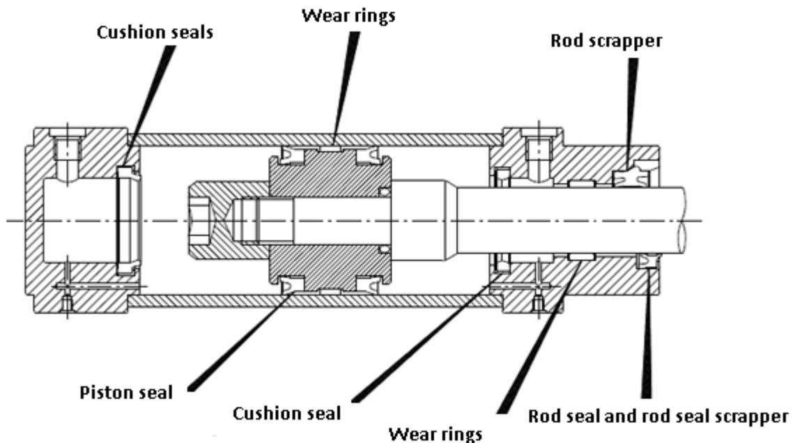
**Figure 1.21** Different types of seals used in pneumatic cylinders
