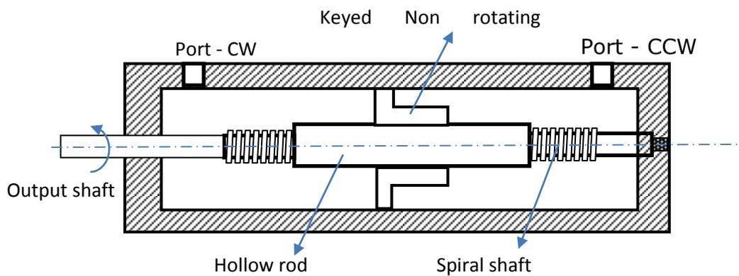
Figure 1.47 Helix spine rotary actuator
