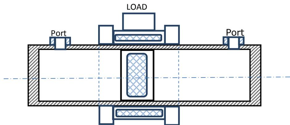
Figure 1.12 Schematic diagram of cylinder with Magnetically Coupled Slide
