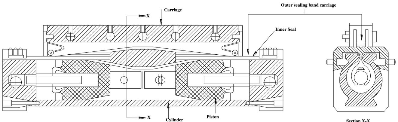
**Figure 1.12** Sealing band cylinder with slotted cylinder barrel
