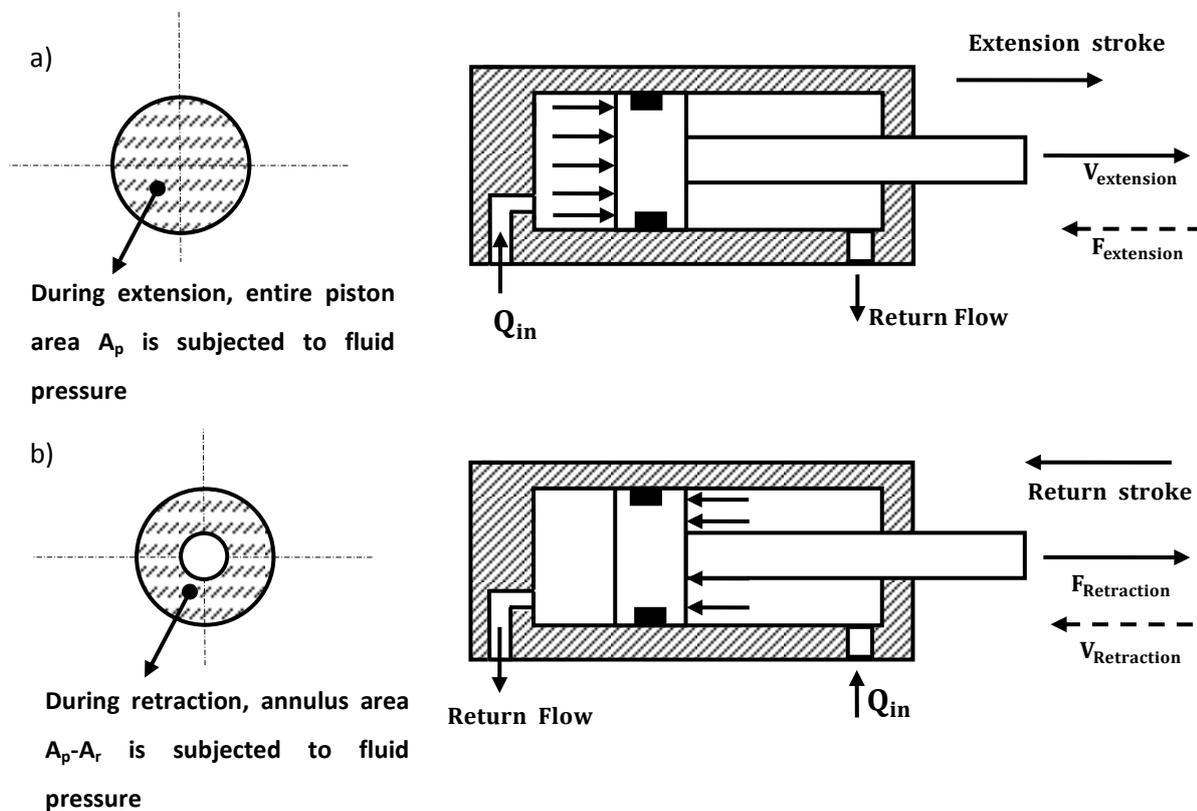
**Figure 1.26** Effective areas during extension and retraction strokes
