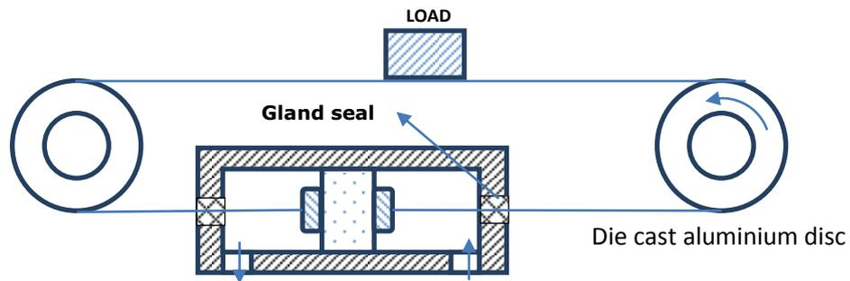
**Figure 1.12** Cable cylinder
