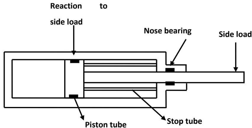
**Figure 1.20** Use of stop tube to minimize side loading.
