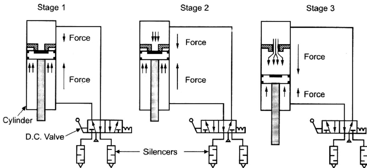
Figure 1.14 Sequence of operation of Impact cylinder
