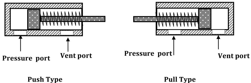
**Figure 1.5 Push and Pull type Single Acting Cylinder**
