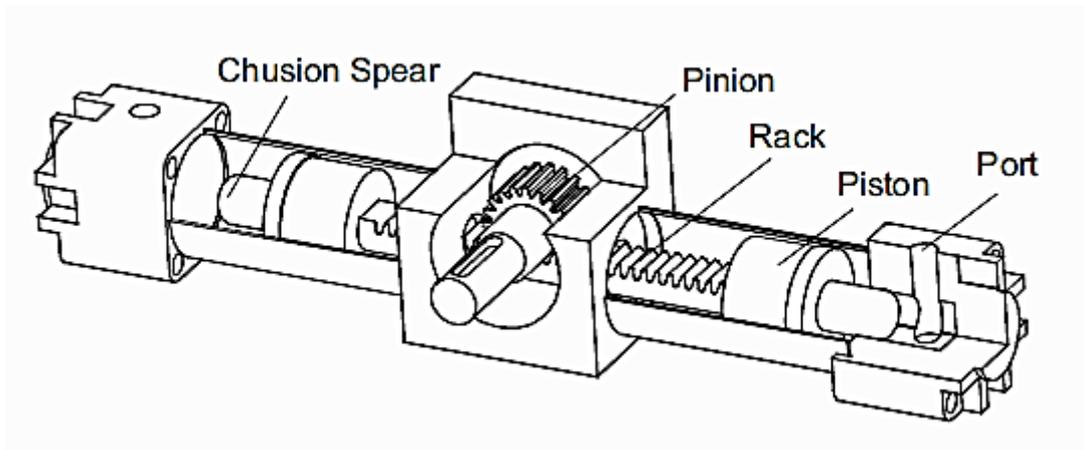
Figure 1.45 Three dimensional view of Rotary Actuator of Rack and Pinion Type
