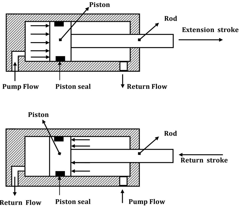
Figure 1.8 Double Acting Cylinder with piston rod on one side
