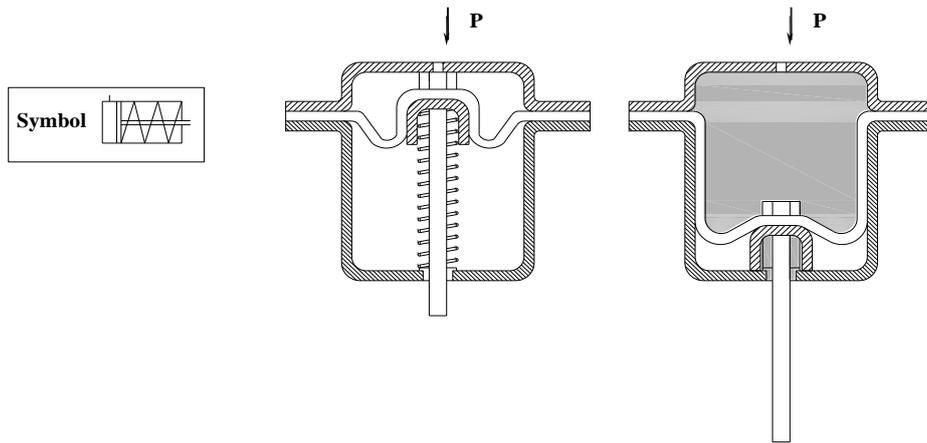
**Figure 1.3** Construction features of rolling diaphragm cylinder
