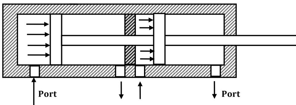
Figure 1.11 Double Acting Cylinder with piston rod on one side
