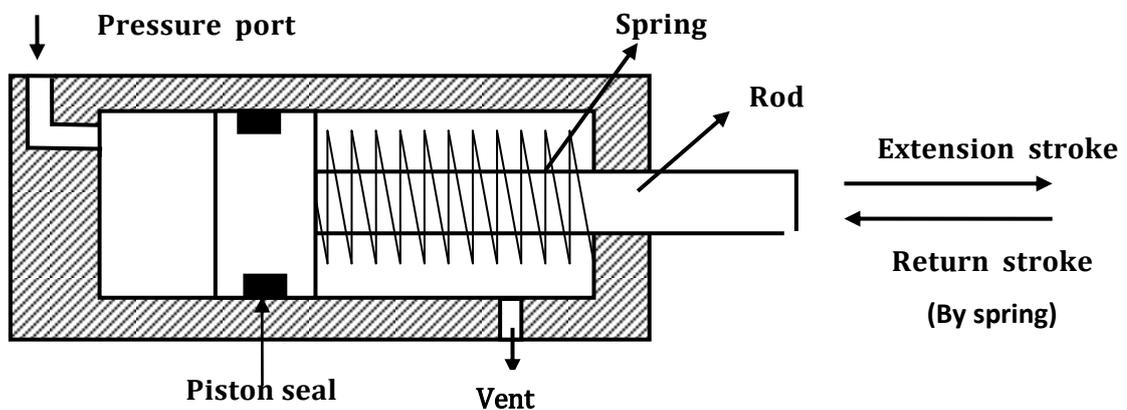
[Figure 1.1](#) Construction features of single acting cylinder
