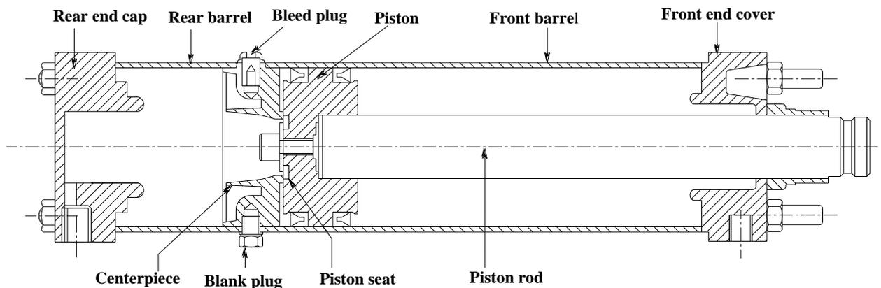
**Figure 1.13 Schematic diagram of Impact cylinder**
