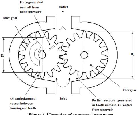
Figure 1.3Operation of an external gear pump
