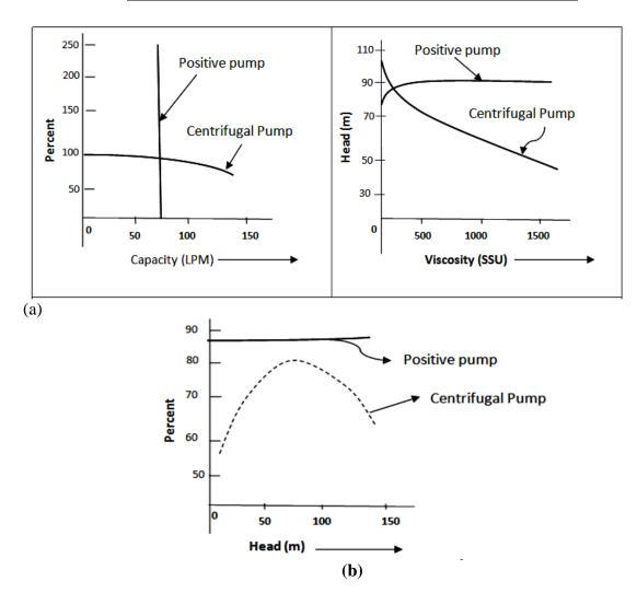
Figure 1.1 Performance curves for positive and non-positive displacement pumps
