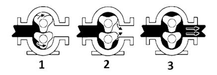
**1.**As the lobes come out of mesh, they create expanding volume on the inlet side of the pump.Liquid flows into the cavity and is trapped by the lobes as they rotate.
