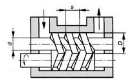
Figure 1.11Volumetric displacement of a screw pump
