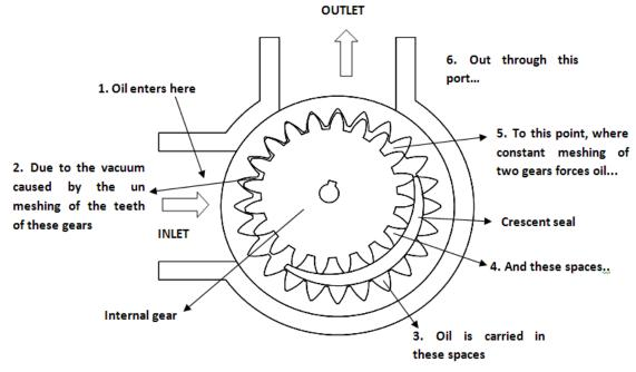
Figure 1.5Operation of an internal gear pump
