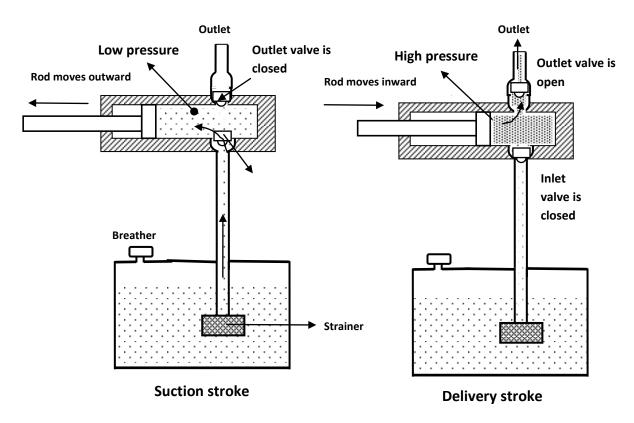
Figure 1.2Illustration of pumping theory
