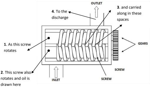
In screw pump, a chamber is formed between thread and housing as shown in Fig.1.11. The following expression gives the volumetric displacement
