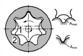
Figure 1.7Gerotor gear pump
