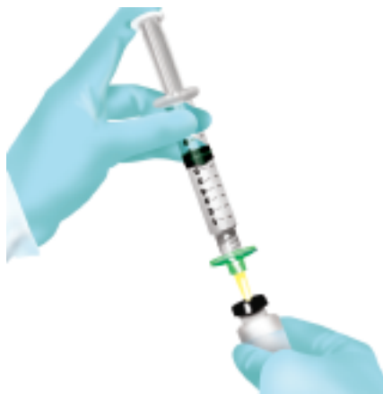
a membrane filter attached to a syringe and needle
