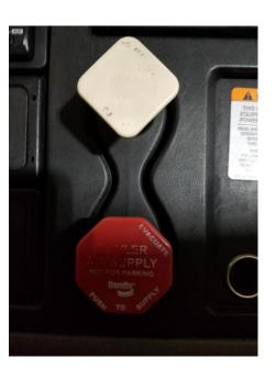
I WILL RELEASE THE PARKING BRAKE BY PUSHING BOTH VALVES IN AND PULL FORWARD TO 5 MPH, DEPRESS THE CLUTCH AND BRAKE WHILE GRIPPING THE STEERING WHEEL TO CHECK IF THE VEHICLE PULLS TO THE LEFT OR THE RIGHT
