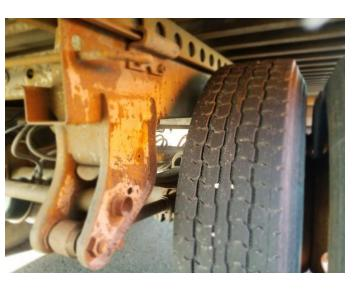
• THE <u>LEAF SPRINGS</u> ARE NOT CRACKED, BROKEN, SCISSORING, OR MISSING
