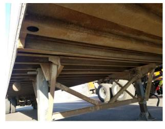
THE <u>FRAME AND CROSS MEMBER</u> ARE NOT BENT OR TWISTED. THERE ARE NO CRACKS OR ILLEGAL WELDS
