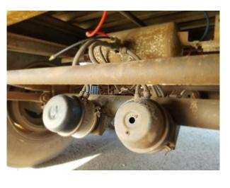
THE <u>AIR HOSE TO THE BRAKE CHAMBER</u> IS SECURELY MOUNTED ON BOTH ENDS. THERE ARE NO SPLITS OR CUTS AND IT IS NOT LEAKING
