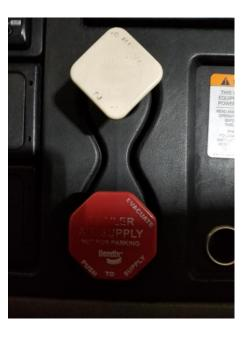
I WILL RELEASE THE PARKING BRAKE BY PUSHING BOTH VALVES IN AND PULL FORWARD TO 5 MPH, DEPRESS THE CLUTCH AND BRAKE WHILE GRIPPING THE STEERING WHEEL WITH BOTH HANDS TO CHECK IF THE VEHICLE PULLS TO THE LEFT OR THE RIGHT
